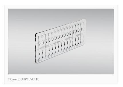
Analytik Jena's CHIPCUVETTE (Figure 1) allows analysis of up to 16 samples in parallel (1 reference and 15 samples). Each sample can be detected with pathlengths of 1 mm and 0.1 mm making dilution redundant.
