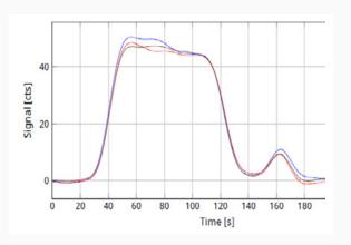
Fig. 6: TN measuring curves for standard 0.5 µg/l N
