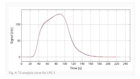
Figure 4 and 5 show the TS analysis curves of both LPG samples. The duration of the measurement depends on the sulfur content and metering volume, and is in average between 150 and 240 seconds.
