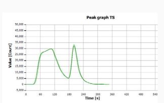
Figure 2: TS determination of "diesel fuel 1" with MPO
