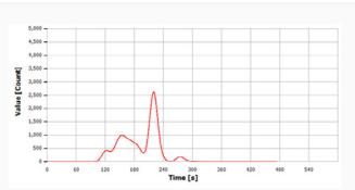
Figure 3: Typical TN measurement curve of maltose
