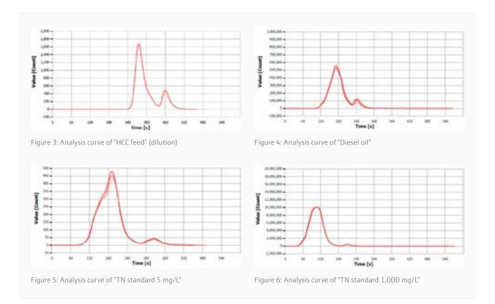
Due to the matrix-optimized combustion in general a threefold determination is sufficient to achieve results far below 3% RSD. This remarkably affects the sample processing time and allows for a higher sample throughput. The analysis results received and their reproducibility prove the performance of the digestion process. The overall performance of the analysis system was validated by analyzing standard materials with known nitrogen contents, results are given in Table 3.
