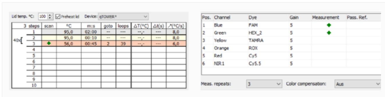
Figure 2: Overview of the settings for bacterial detection in qPCRsoft for the real-time PCR on the qTOWER<sup>3</sup>. The target DNA is detected in the blue channel, while the internal control is detected in the green channel.
