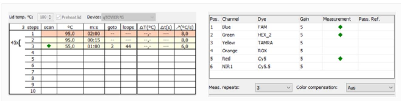
Figure 3: Overview of the settings for *Legionella* detection in qPCRsoft for the real-time PCR on the qTOWER<sup>3</sup>. *Legionella pneumophila* and *Legionella spp.* can be detected in the blue and red channel, respectively. In the green channel the internal control can be detected.
