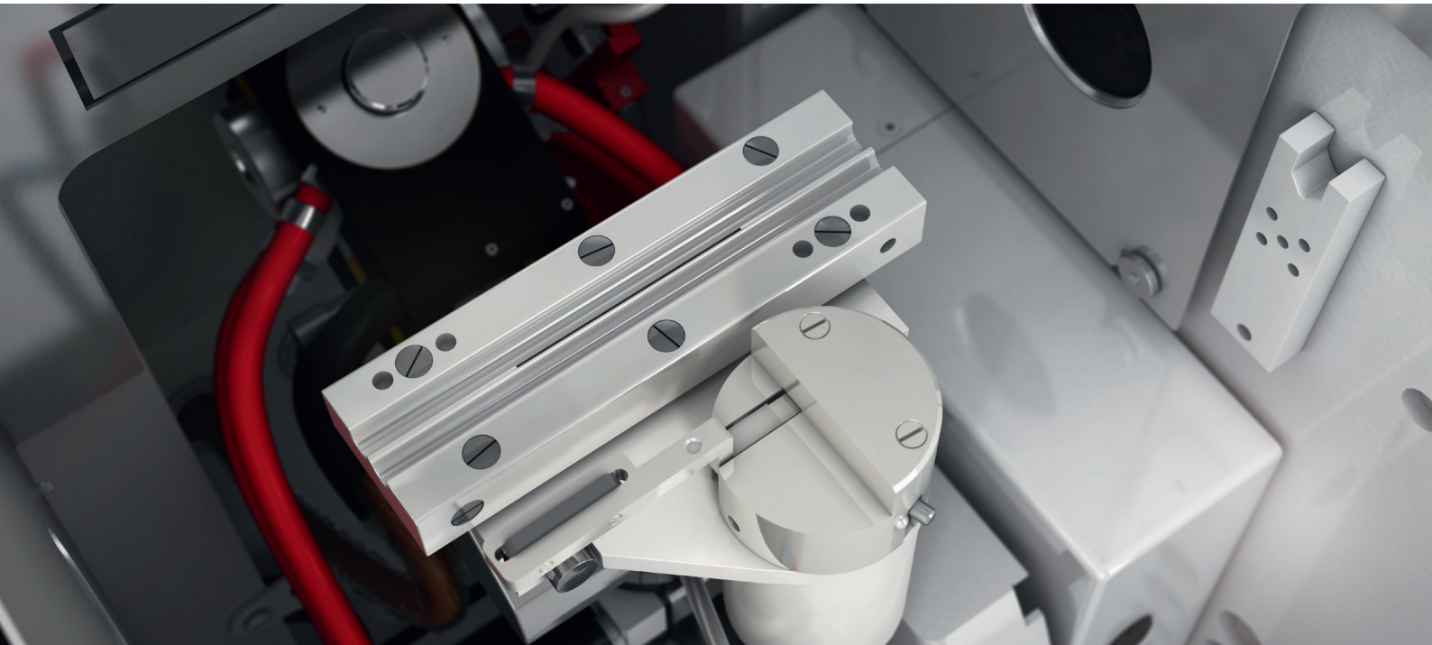
Burner head with Scraper and lowered graphite furnace (novAA 800 D)
